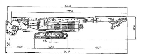
Massa /Weight (mast base + PDW 2m + 3 m) ~ 91000 kg
