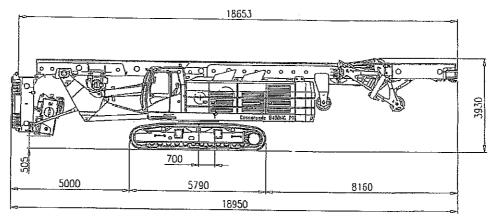
Massa/Weight (mast base + PDW 2m + 3 m + 3 m) ~ 92000 kg
