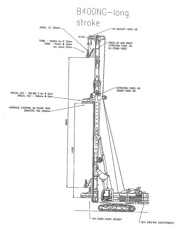
weight of base machine + mast, without rotary heads and counterweight: 78t
